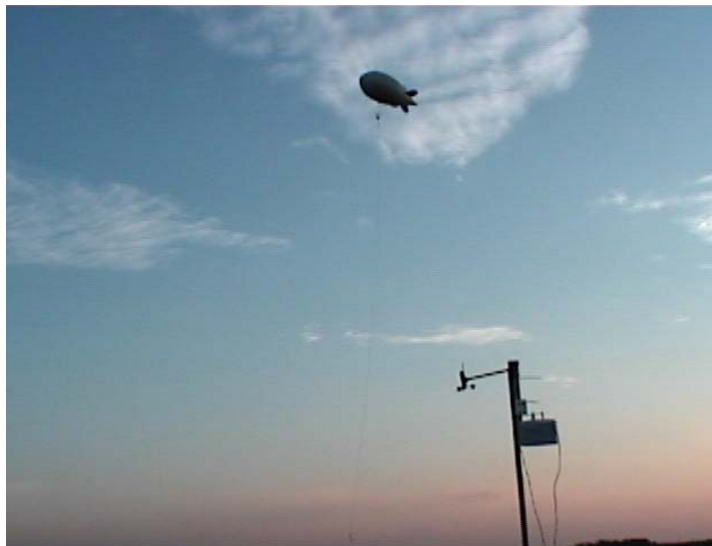
Meteorological data during the spraying/sampling period was recorded both at flight altitude with a kiteon and at ground level with a weather station.
